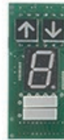
Seven-Segment-Code Segment display: vertical display Display color: red Input voltage: DC 24V Parallel Input signal: 7 Segment Function display: overload, inspection
