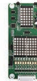
Dot-Matrix display, vertical display Display color: red Input voltage: DC 24V Parallel Input signal: BCD code, Gray code Function display: overload, inspection
